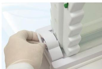
6. With the cam pin handles facing directly downwards, turn the cam pins fully through 135° or until the insert has tightened onto the silicone mat.
