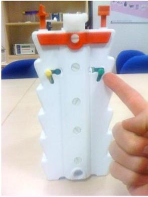
1. To replace the green sliding gel clamps, begin by unscrewing the colour-coded vertical screw pins. There should be no glass plates within the PAGE insert, in the side(s) being unscrewed. Once the screw pins are unscrewed sufficiently the green clamp should sit in the resting slot as shown.
