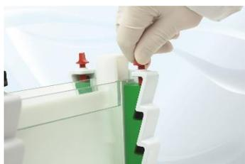
3. Fully tighten the screws, making sure not to wobble the unit.
