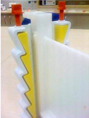
6. Withdraw the sliding gel clamps so that they sit suspended in the resting slots as shown. Repeat steps 1-6 to replace the remaining green sliding gel clamps. Once complete the PAGE insert is ready for 4-gel assembly.
