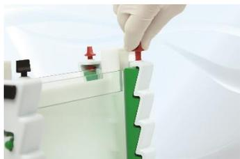
2. Position the Slab Gel Insert on a flat surface. Insert the glass plates into the Slab Gel Insert between the clamps and the white gasket. The Slab Gel Insert contains clamps which impart even pressure onto the glass plates and allow even screw pressure transfer onto the sealing edge of the glass plate, ensuring complete sealing.
