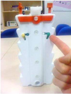
2. Gently push the green sliding clamp horizontally towards the core of PAGE insert until it can move no further.
