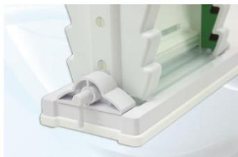
5. Position the Slab Gel Insert in the casting base such that the Cam pins have handles pointing downwards and are located in the insert holes. The top of the module may need to be pushed down very slightly to locate the cam pins.
